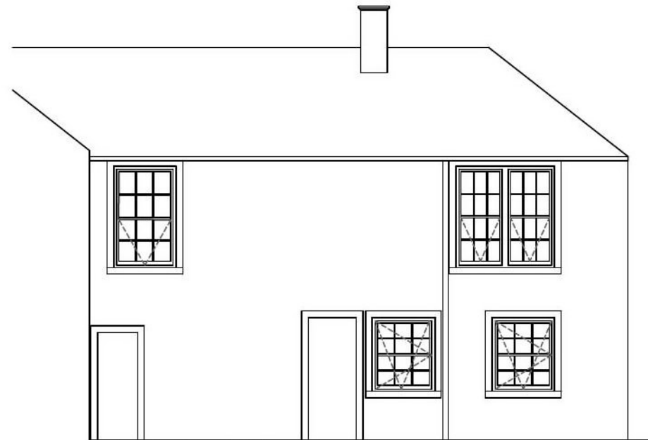
North Elevation (Side) Proposed UPVC Casement windows in green to match existing
